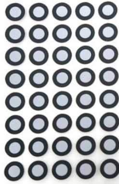
Figure 7-6 Markers With 6mm Inner Diameter And 10mm Outer Diameter
