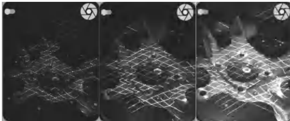
Figure 7-12 Brightness of Laser Line-Underexposed/Moderate/Overexposed
