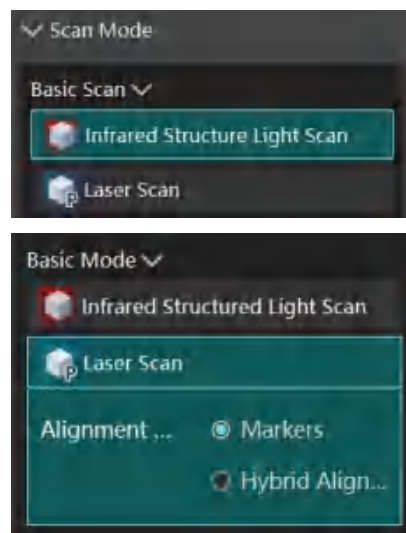
Figure 7-1 Two Basic Scan Modes of 3DeVOK MQ
