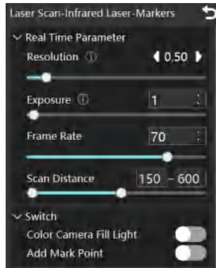
Figure 7-9 Infrared Laser Settings in Marker Mode
