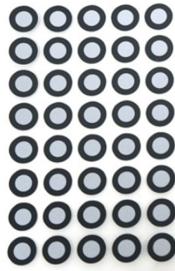
Figure 7-5 Markers With 6mm Inner Diameter And 10mm Outer Diameter (Unit: mm)
