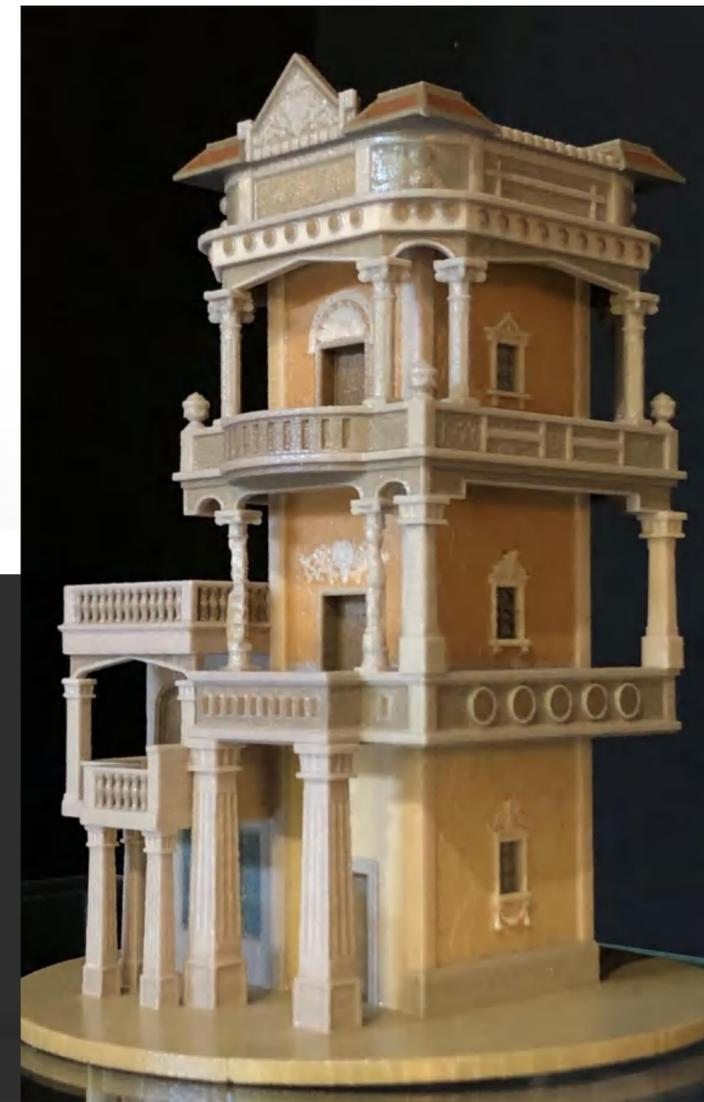
Field study → Partial scanning of buildings → Data processing (forward + reverse) → 3D printing
