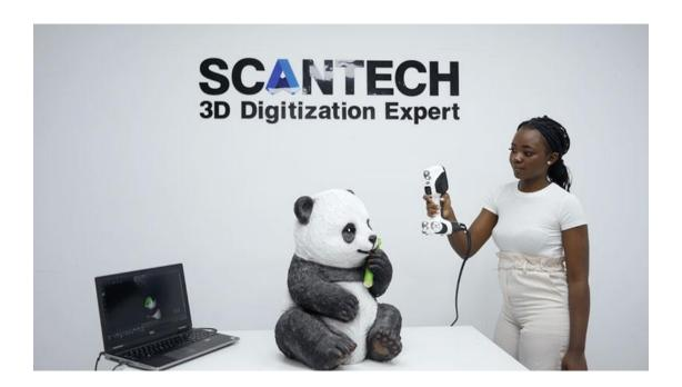
Note: Scanning powder is required for iReal 2E when scanning transparent, specular, and euphotic materials. Industrial laser scanners from Scantech can easily deal with the dark and reflective surfaces without powder and get high-quality point clouds.
