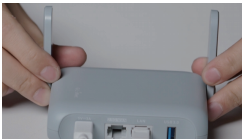
Figure 1-3 Transceiver Antenna Deployment
