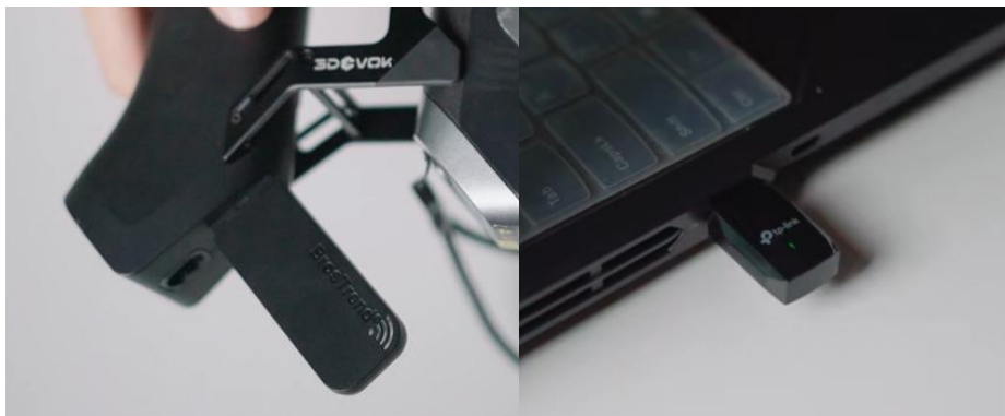
Figure 3-14 Assembly of the Primary Network Card and the Receiver
