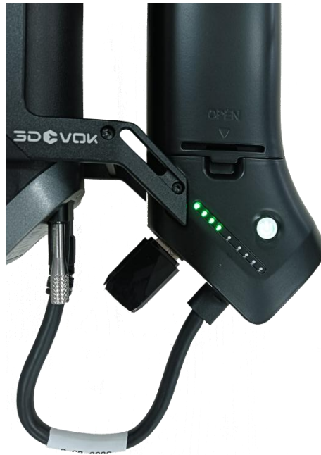
Figure 4-15 Central Indicator Light Being Off
