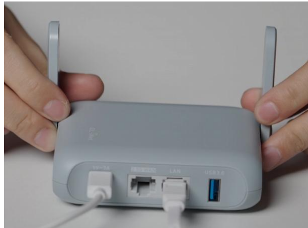
Figure 3-6 Transceiver Antenna Deployment
