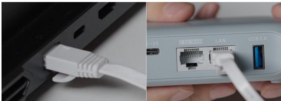
Figure 3-4 Router's Ethernet Cable Connection
