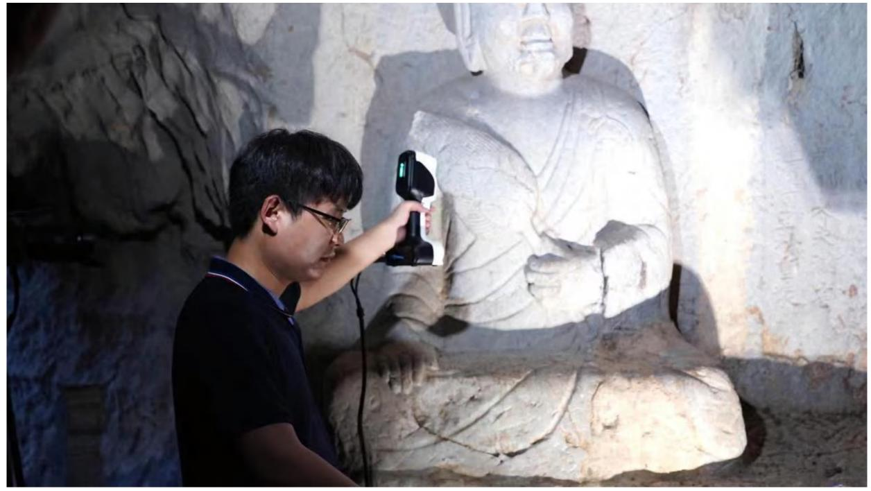
3D scanner: iReal 2E; Highest accuracy: 0.1 mm; Highest resolution: 0.2 mm
